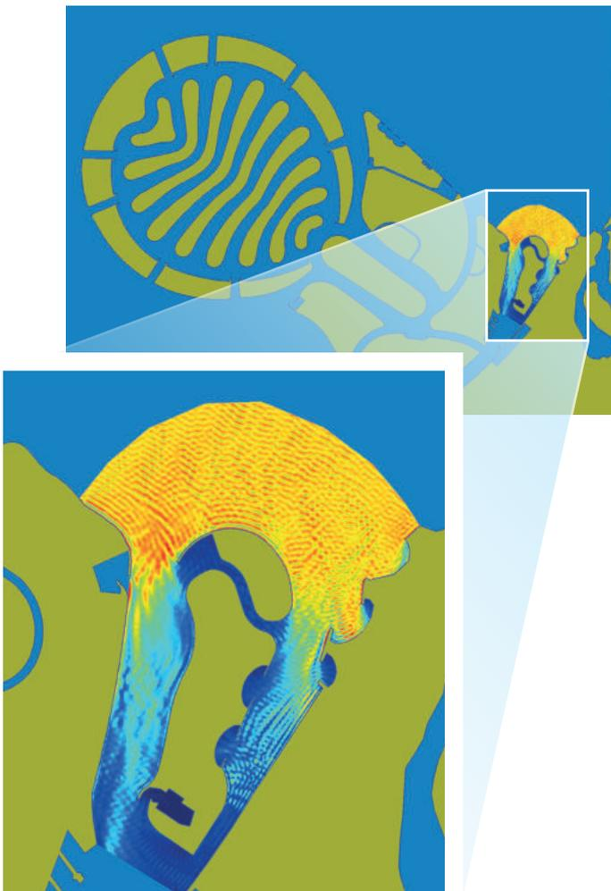
Wave height pattern resulting from a PHAROS directional spreading computation. Palm Deira, U.A.E
