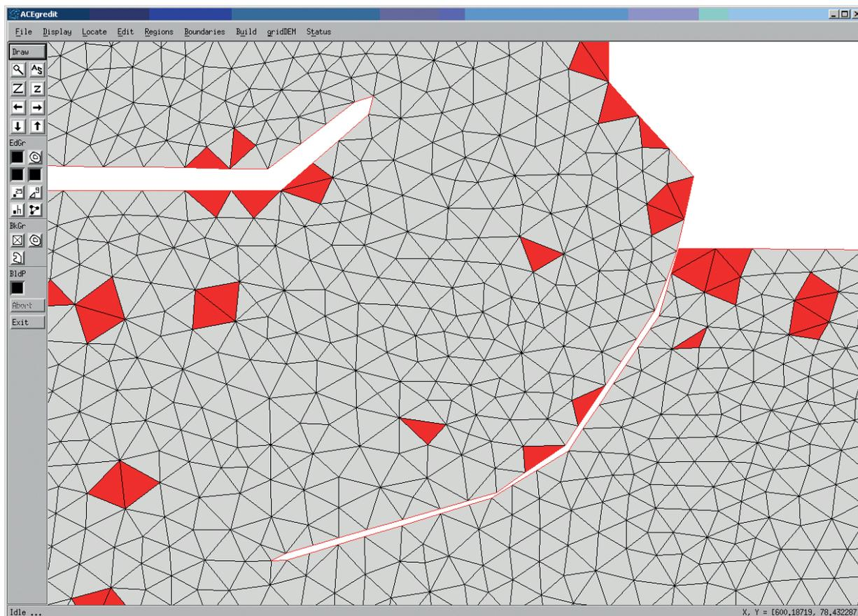
Detail of a PHAROS computational grid. In red the computational elements that are too large for the local wave length.
