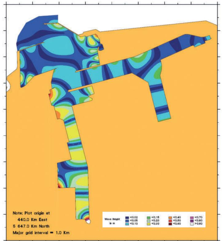
Example of harbour resonance simulation for the Port of Dunkerque: amplification at selected points as a function of the frequency (insert) and wave height pattern for the highest peak.
