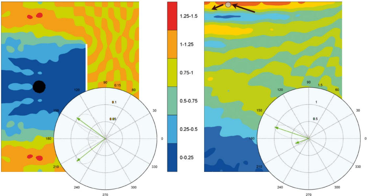
Applications of the PHAROS wave direction post-processing tool. (Left: Sheltering behind a breakwater; Right: Partial reflection)
