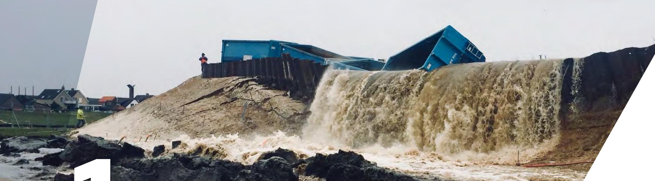
*'We collected data in this trial to make it clear how steel sheet piling really works in a dike during high water. That will be a great help in any event on dike upgrades in the future!'*
