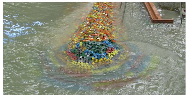
Testing a breakwater model and studying the wave climate
