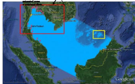
Figure 3.1 Computational grid (flexible mesh) overview. Pins show the locations of all tidal stations. Horizontal resolutions of 8000m, 4000m and 2000m are noticeable. The red rectangle indicates the zoom level shown
