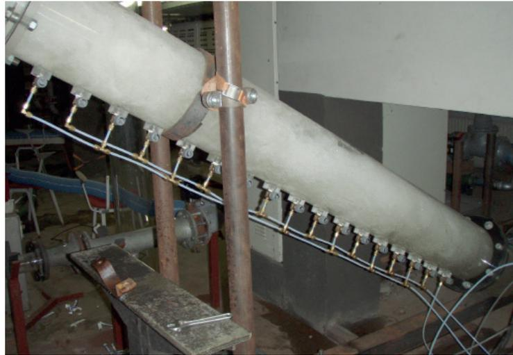
Pressure measurement in a gas-entraining hydraulic jump
