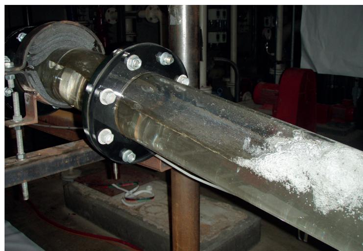
Hydraulic jump demonstrated in a transparent pipe sections
